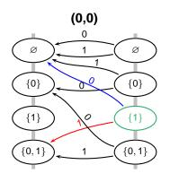
$$B_{00} = \left[ \begin{array}{ccc} 1 & 0 & 1 \\ 0 & 0 & 0 \\ 0 & 1 & 1 \end{array} \right].$$
